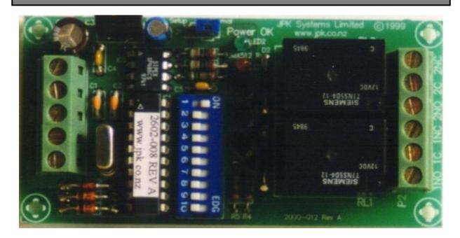
DMX contactor boards by JPK Systems Ltd provide both normally open and normally closed isolated contacts capable of switching low current signals and high current power loads. Integration of existing equipment into a DMX512 lighting control system is easy and cost effective.
